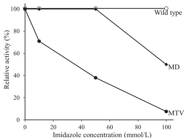
Fig. 5 Effects of imidazole on the enzyme activities. Approximately 0.3–40  $\mu\text{g}/\text{mL}$  of each enzyme in a reaction mixture was assayed. Open circle, closed rhombus, and closed circle indicate wild-type, MD, and MTV, respectively.
