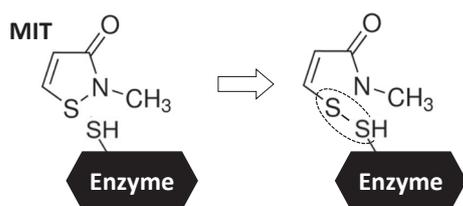
Fig. 2. Chemical modification of thiol groups in enzymes with *N*-methylisothiazolinone (MIT).
